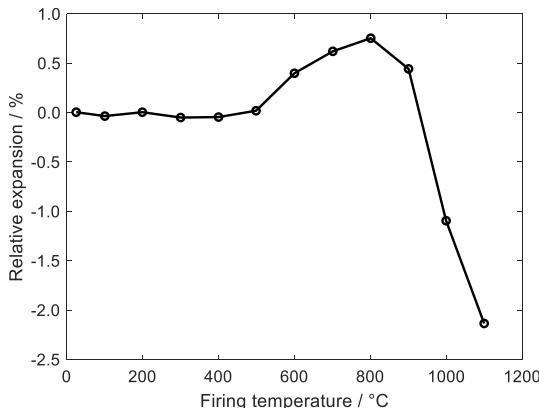
**Figure 3:** Relative expansion of the clay sample after firing at different temperatures
