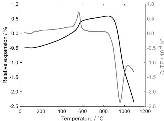
**Figure 1:** Thermodilatometric curve (black line) and CLTE (gray line) of the unfired sample during heating to 1100 °C at 5 °C/min
