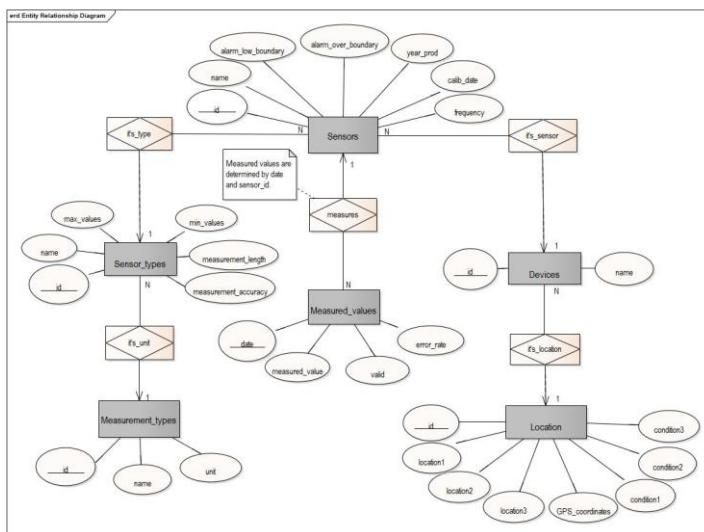
**Figure 1:** Entity relationship diagram of our database
