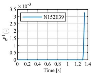
**Figure 7:** Accumulated plastic strain time-history curve at node N152E39
