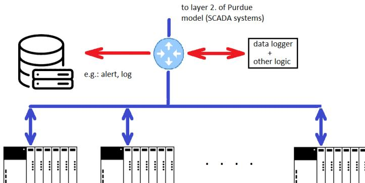
**Figure 4:** The (part)architecture of industrial network and data logger with other reconfigurable module
