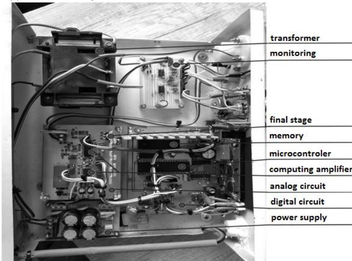
Fig.3 Designed electronic instrument as teaching aid
