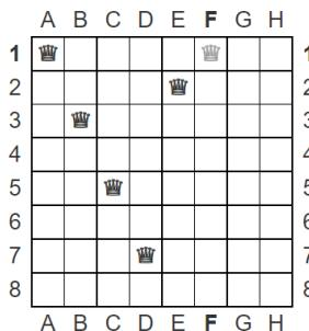
**Figure 2:** Backtrack algorithm visualization: Eight queens puzzle with already placed queens and the currently investigated newly added queen
