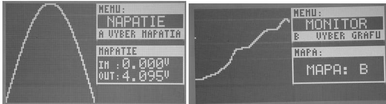
**Fig.5** Graphical imaging of transfer characteristics including possibilities to display other parameters
