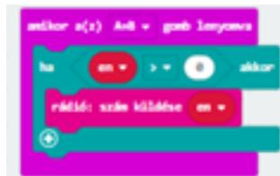
**Figure 4:** “on button A+B pressed” method
