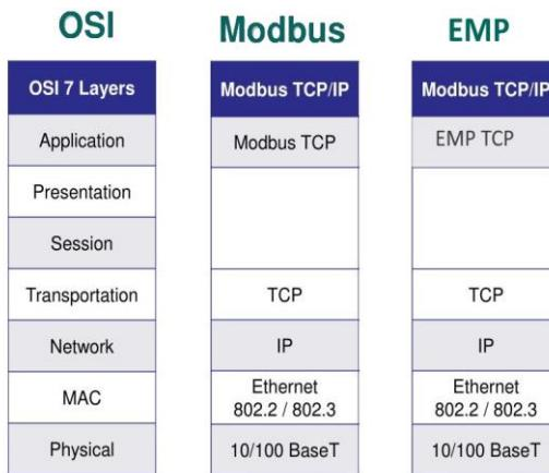
**Figure 4:** Layers of OSI, Modbus TCP and Own protocol
