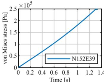
**Figure 9:** von Mises stress time-history curve at node N152E39
