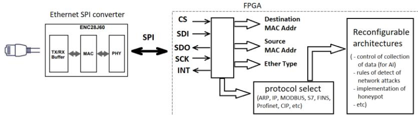
**Figure 3:** The scheme of architecture of datalogger
