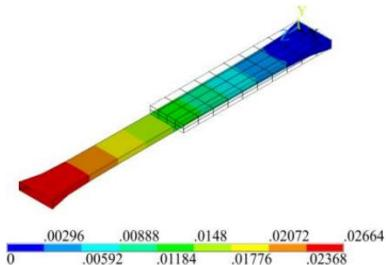
**Figure 4:** Axial displacement distribution [m] at the end of the analysis
