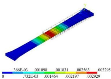
**Figure 6:** Accumulated plastic strain distribution [-] at the end of the analysis
