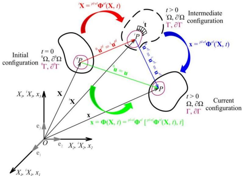
**Figure 1:** The proper kinematics of finite elastoplastic deformation
