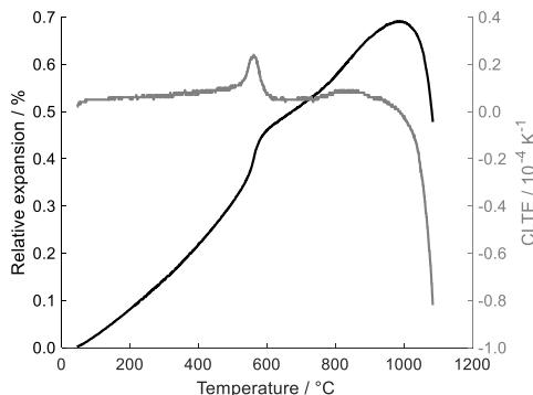
**Figure 2:** The relative expansion (black line) and CLTE (gray line) of the clay fired at 1100 °C
