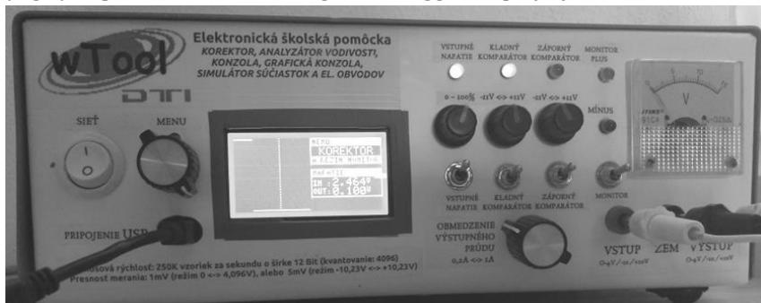
**Fig.6** Front panel of designed teaching aid including built-in display
