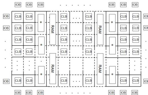
**Figure 2:** The scheme of FPGA
