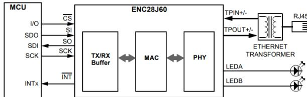
**Figure 1:** The scheme of ENC28J60 device [3]
