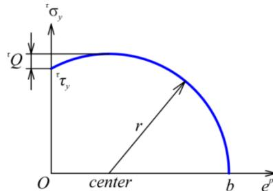
**Figure 2:** The yield stress versus uniaxial plastic strain curve of the material
