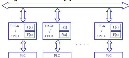
**Figure 2:** PLCs and Programmable Logic Circuit (FPGA or CPLD) with encryption and decryption algorithms
