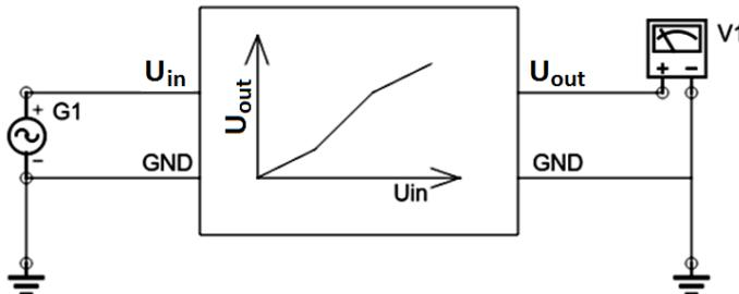
**Fig.1** Principle of designed electronic teaching aid
