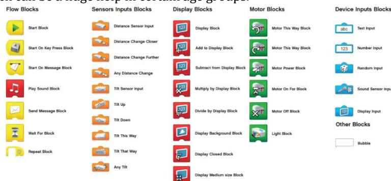
Figure 2: The programming blocks of WeDo 2.0
