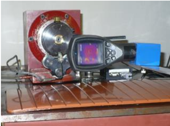
Fig. 3: Monitoring of the temperature of the sliding joint using a thermocouple and thermal camera
